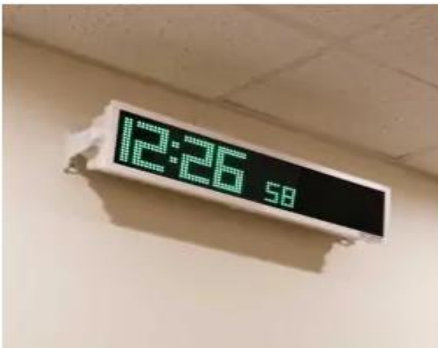
Figure 2: Modern Wireless LED Message Board: For Text Messaging and Digital Time Display
