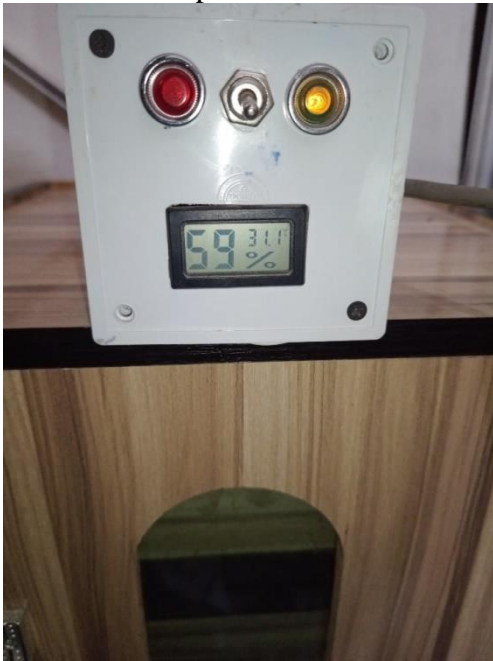
Fig. 1. The control box shows the power ON/OFF switch with the L.C.D. display.
