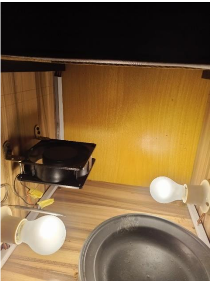
Fig. 7. The bulbs are used to provide heat to the system, while the fan is used to spray the heat across and also help in regulating the temperature of the whole system.
