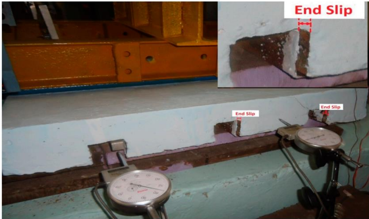
Figure 9. Slip of rectangular profiled composite decks
