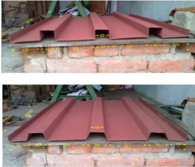
Figure 4. Dovetailed, rectangular, and trapezoidal profiled sheet (All the dimensions are in mm)
